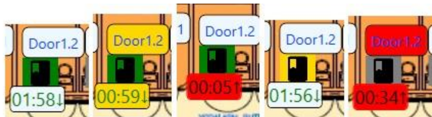
Example of Alert Count Down Function (white: alert triggered, yellow: alert in action, red: alert in warning state)
